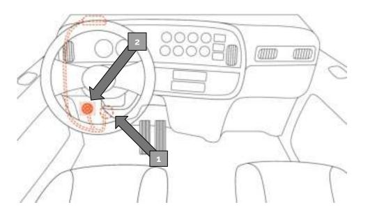
Attach the other side of the cable to the Cartrack ELD.
