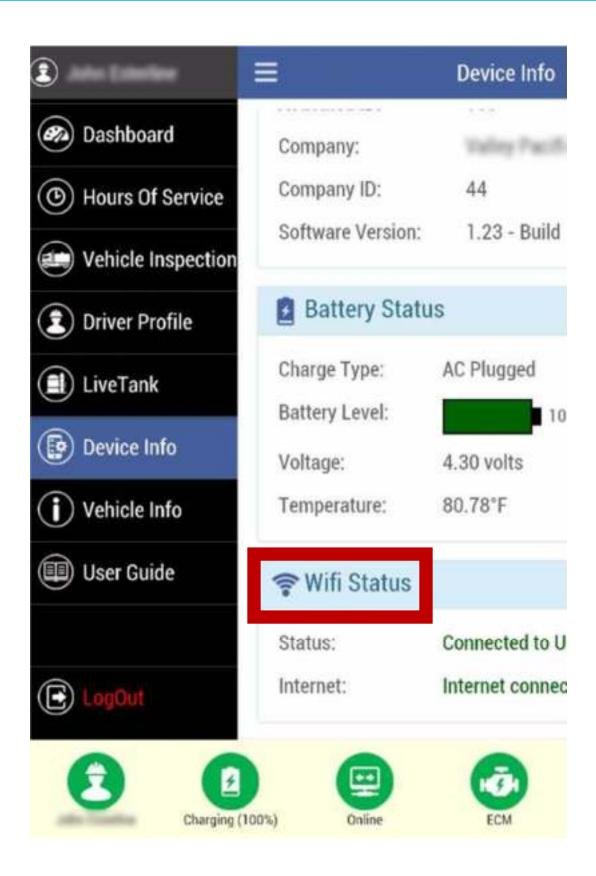
Symptom: [ECM] icon shows in "red", ELD may have lost connection to vehicle ECM (Engine Control Module). Try the following:
