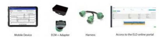
Your mobile device (where the ELD app is running) must a) have Bluetooth enabled and b) be connected to the internet either with a cellular data plan or connected to a hot spot.
