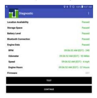
Bluetooth and ECM connection status: The ELD must be able to read engine data at all times. Make sure the Bluetooth and ECM connection indicators remain green. If the indicator turns red, please go to Scan Devices and connect to the ECM-linked device.
