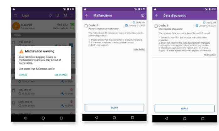
When you see the malfunction indicator, you should view the malfunction details by tapping the indicator. This opens the 'Malfunctions' screen that lists malfunction events recorded on the ELD. You can view the details of a malfunction and clear it.
